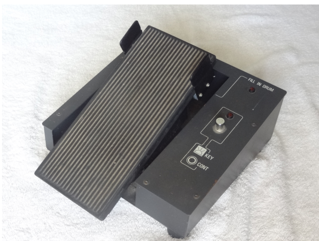
Figure 3: Expression pedal from an Excelsior Digiszyzer (c1980) hybrid accordion showing dual toe-switches.
